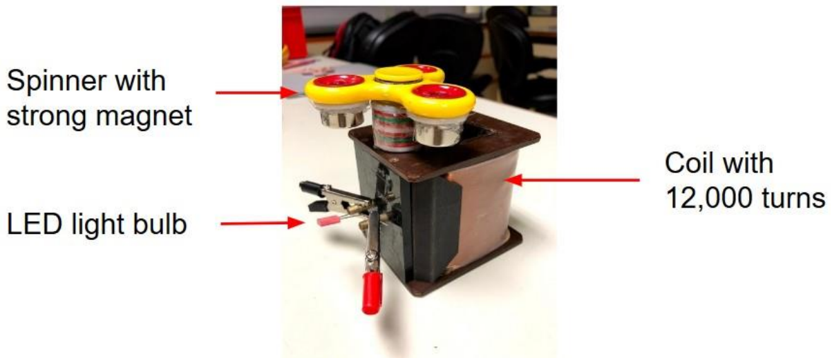
Figure 2: Experimental set-up for the demonstration on Faraday's Law
