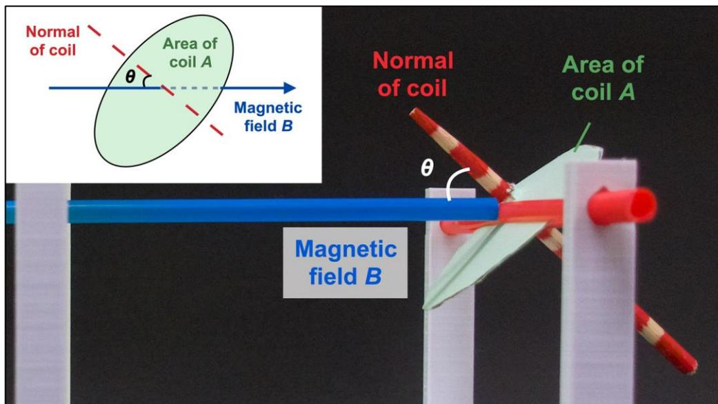
Fig. 1 The 3D Magnetic Flux model
